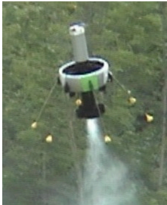
Fig. 7 Georgia Tech's HeliSpy (GTSpy) 11 inch ducted-fan UAV.
